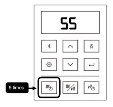
Service Soon (SS) will display on the controller again when the boiler reaches the interval selected in the parameter settings.
