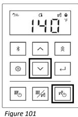
While continuing to hold the (Down) button, press and hold the **Domestic Hot Water** button (press and hold both buttons down at the same time).
