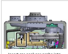
Insert gas analyzer probe into combustion analysis port.
