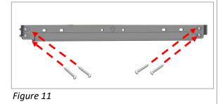
Insert the top bracket into the wall mounting bracket. Make sure the wall mounting bracket is attached to the wall and can hold the weight of the boiler before you fully let go.
